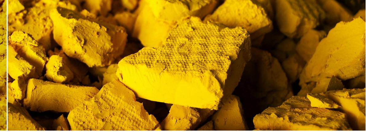
Yellowcake is the intermediary. It is produced through the in situ leaching of acids into boreholes drilled into a mineral deposit. Yellowcake is rarely yellow. This was simply the colour associated with early extraction efforts; the process is now more efficient. Yellowcake is what remains after drying,
